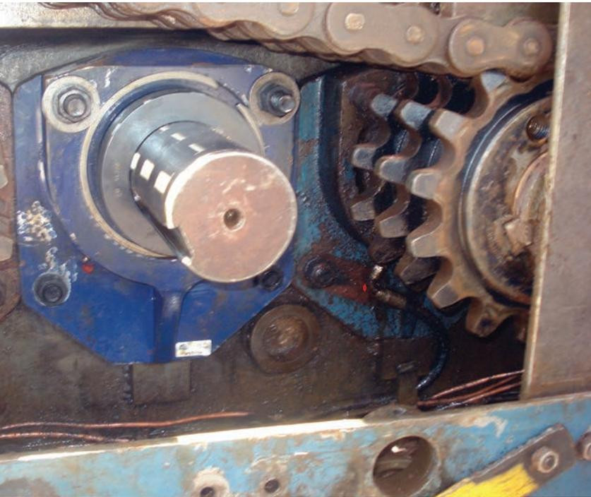
Still operating seven months later, the Timken flange block continues to work like new. The triple-lip seal keeps contaminants out and is proving to be superior to the competing bearing. The unit handles more than two times the weight of the old bearing, with an expected design life of 100,000 hours.
