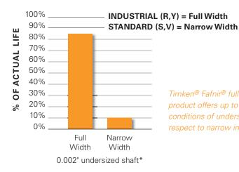
Timken® Fafnir® full width inner ring product offers up to 8 times life in conditions of undersized shafting with respect to narrow inner ring product.
