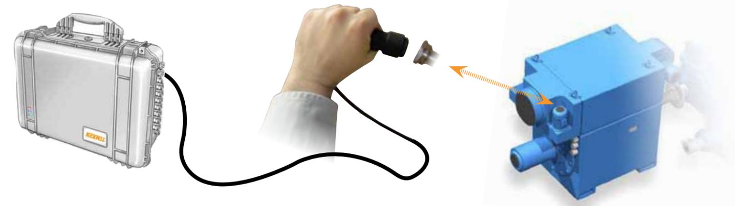
Timken's portable Online Intelligence System uses the same technology as the Online Intelligence System, but the portable option is designed for field troubleshooting and temporary installations. The portable system is packaged in a rugged plastic enclosure with external sensor connections, making it perfect for Timken's field services group to support your installations.
