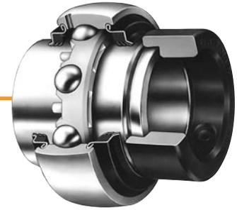
Timken® Fafnir® is found in a wide array of ball bearing applications. Each bearing is designed with the same idea in mind – to maximize performance. The original wide inner ring ball bearing provides customers with a product that is easily mounted on straight shafts and positioned without shoulders, locknuts or adapters. This same design is still preferred in farm equipment applications.
