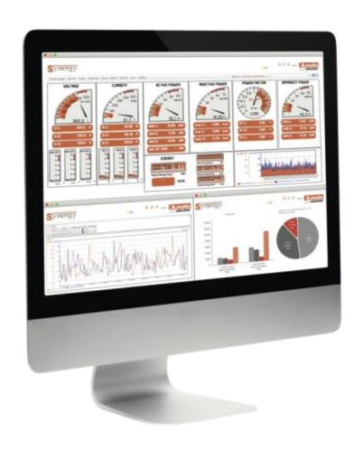
Synergy is upgraded with important functions which increase flexibility in use. The possibility of integrating third party devices - provided that they are able to communicate through Modbus protocol - has been added.
