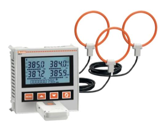
The DMG611 multimeter is a measuring device with four voltage inputs (three phase and neutral) and three inputs for reading the phase currents through Rogowski coils. The main advantage of these coils is their flexibility and deformability, so that they are highly suitable for system retrofitting. The built-in RS485 communication port enables the inclusion of DMG611 in a supervision network. The multimeter is compatible with the Synergy and Xpress software and with the App SAM1.
