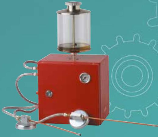
The liquid flows from the reservoir into a piston pump. This pushes an exact quantity of the lubricant into the internal feed tube. Separately supplied compressed air splits the medium at the nozzle tip and sprays it. External MQL in all metal-cutting operations. Pinpoint or small area lubrication in chipless forming operations. Application of mould release and anti-corrosion agents or other spray-on substances.
