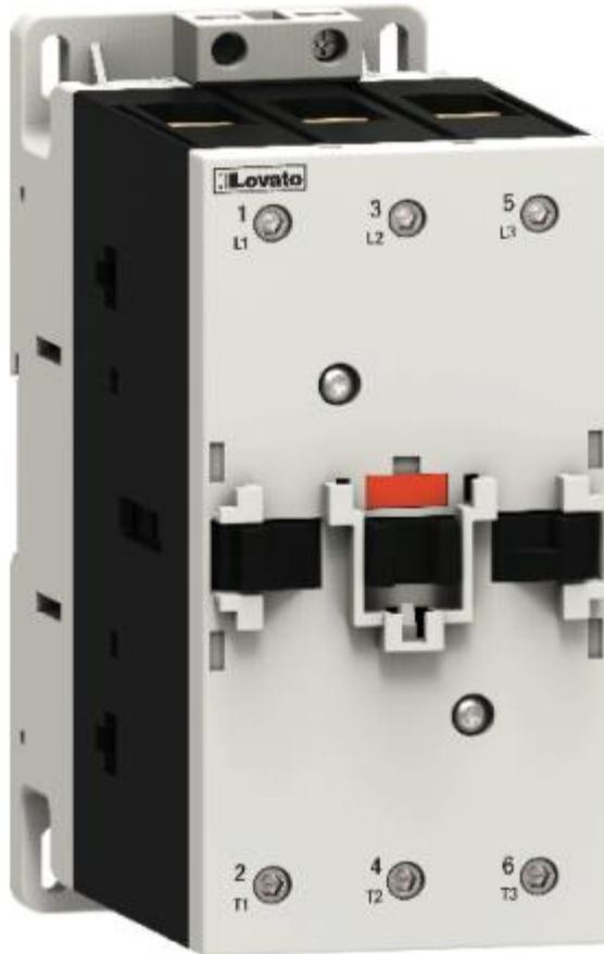
They have a small footprint: 75mm for the three-pole versions and 100mm for the four-pole versions. Motor currents at 400V from 95 to 150A and thermal currents  $I_{th}$  from 140 to 165A.
