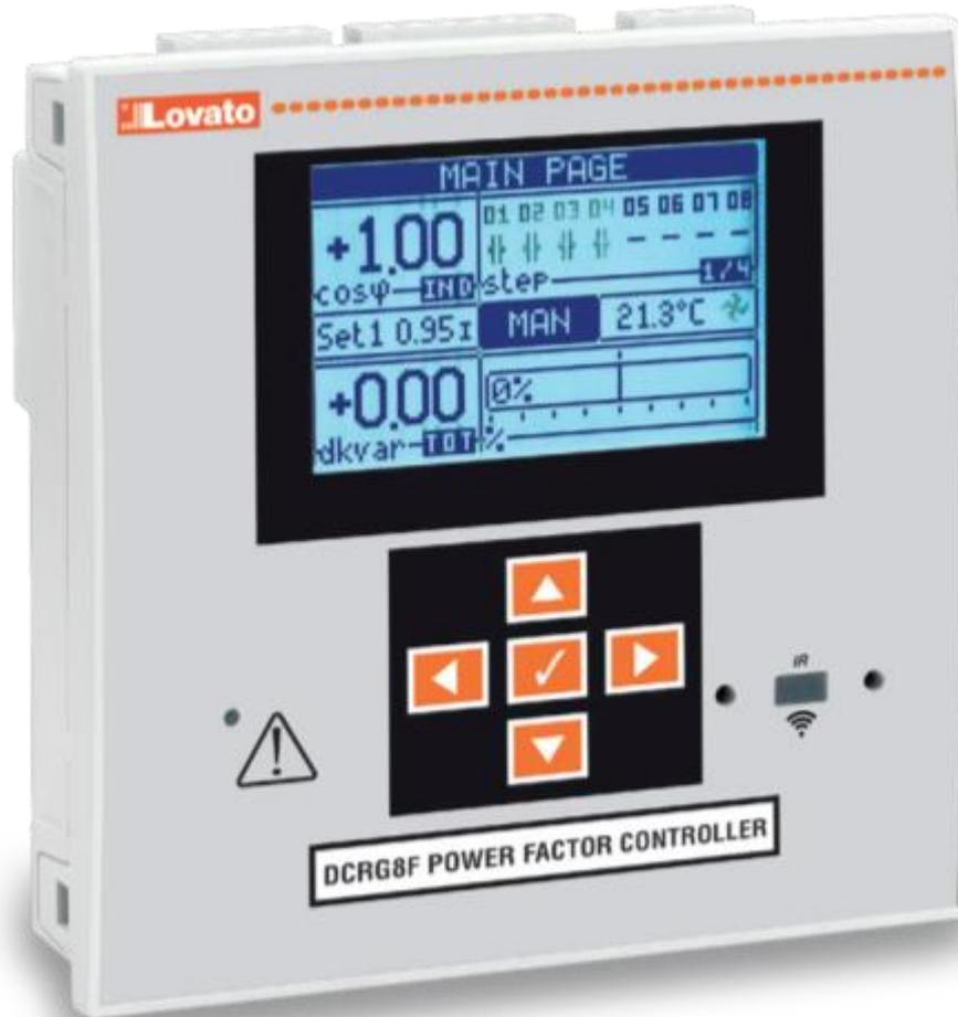
It has been designed to control power factor correction panels with steps added through thyristor modules, particularly suitable for systems with inductive loads that change very quickly over time.
