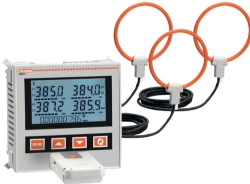
The DMG611 multimeter is a measuring device with four voltage inputs (three phase and neutral) and three inputs for reading the phase currents through Rogowski coils. The main advantage of these coils is their flexibility and deformability, so that they are highly suitable for system retrofitting.
