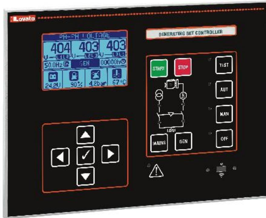
RGK750 is the new LOVATO Electric generating set controller with black front cover, graphic display, AMF (Automatic Mains Failure) management and advanced features as the buzzer for alarm notification, the remote alarm output for RGKRR support and built-in PLC. Two slots can host EXP expansion modules which let the controller to be equipped with communication options or additional digital inputs and outputs. Canbus J1939 is available on board.
